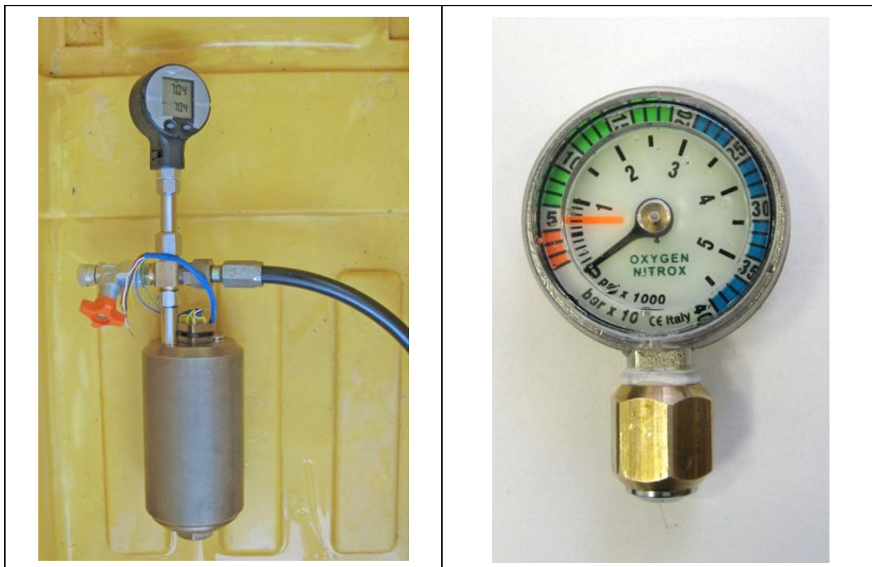
Figure 5 Test process at left and the pressure indicator after the test without any signs of failure.
