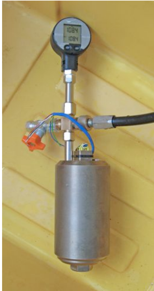
Figure 7 Test in progress. Indicator under test is being pressurised to 110 bar, where it was held for 15 minutes.
