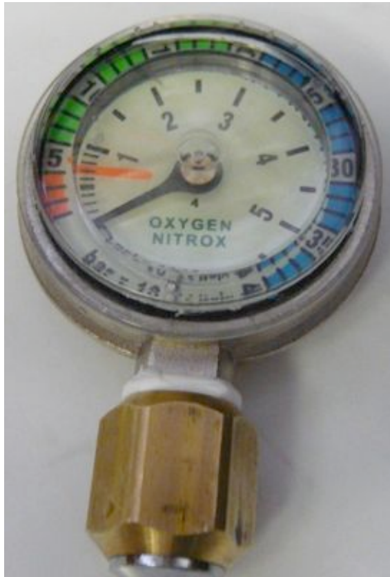
Figure 6 Pressure indicator after the test with crack on the glass (top side of the image). There was no water entry into the pressure indicator.
